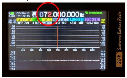
2. Adjust the highlight to the section shown in the image below and switch the setting to 'STE 192k'
