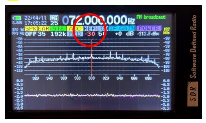
5. Adjust the highlight to the section shown in the image below (IF GAIN) and switch the setting to '+0 dB'
