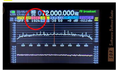
3. Adjust the highlight to the section shown in the image below (AGC) and switch the setting to 'AGC-MID'
