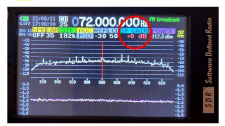
6. Adjust the highlight to the section shown in the image below and switch the setting to '-10, 0KHz, 10'
