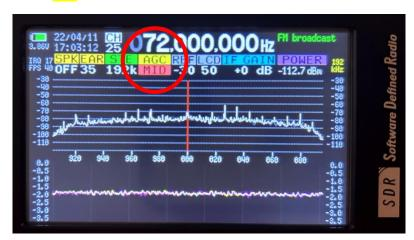
4. Adjust the highlight to the section shown in the image below (REF) and switch the setting to '-30'
