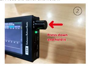
3. Hold the tuner and spin for the adjustment setting
